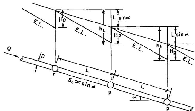
FIG. 1. Pipeline with Equally Spaced Pumping Units
