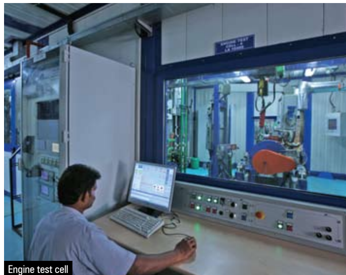
Engine test cell
