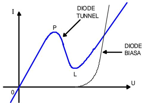
Gambar 2.110 Karakteristik  $I = f ( U )$  Dioda Tunnel
