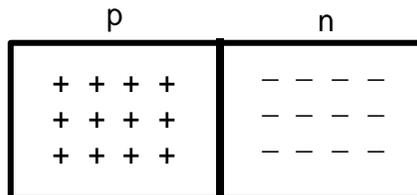
Gambar 2.89 Dioda Junction
