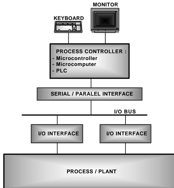
Gambar 1-3: Sistem Otomasi *Direct Digital Control* ( DDC ) [1]
