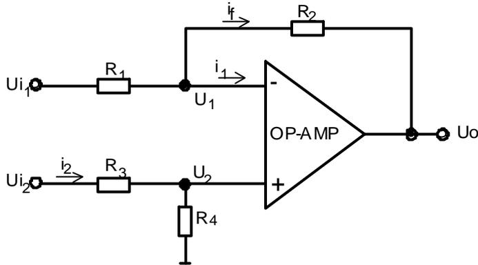
Gambar 2.230 Rangkaian "Subtractor"
