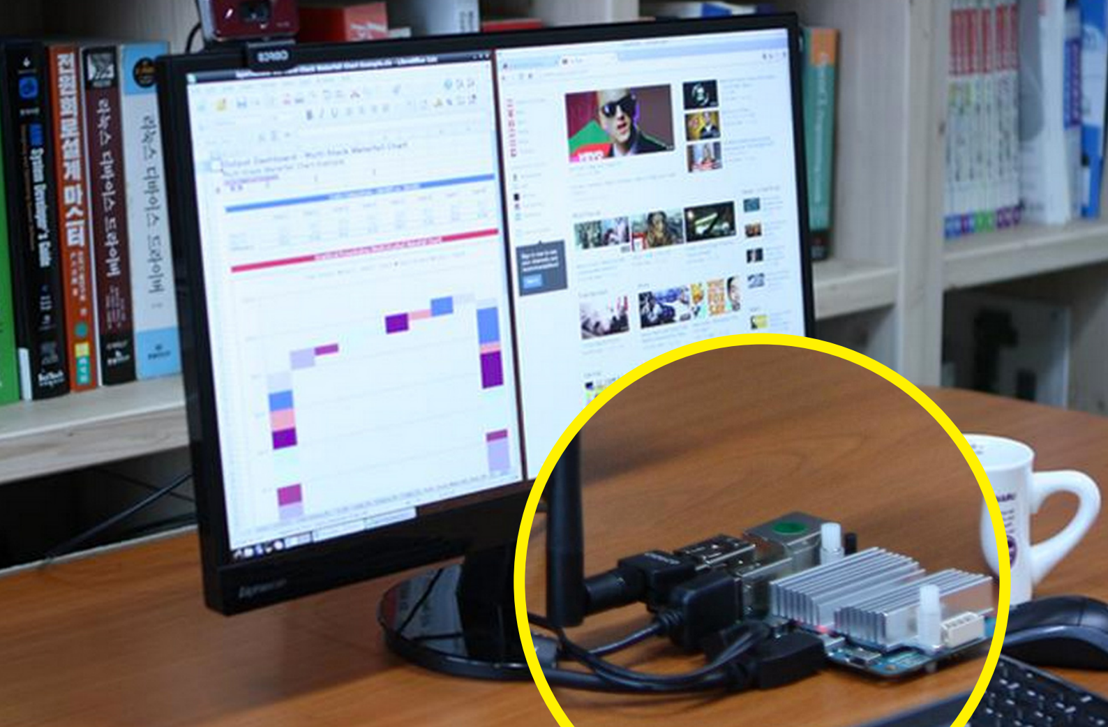
A typical ODROID-U3 setup. A 21-inch monitor is connected to the HDMI port, and the keyboard, mouse, WiFi and USB camera are connected to 3 USB ports.
