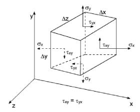
So if we take the xy plane then  $\sigma_x$ ,  $\sigma_y$ ,  $\tau_{xy}$  will be the only stress components acting on the parallepiped. This combination of stress components is called the plane stress situation
