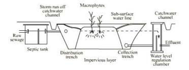
Aquatic plant ponds consisting of free floating macrophytes, such as water hyacinths, duckweeds, etc. have been cultured in ponds either for their ability to remove heavy metals, phenols, nutrients, etc. from wastewaters or to assist in giving further treatment to pretreated wastewaters to meet stringent discharge standards while at the same time producing new plant growths for their gas production or food value.
