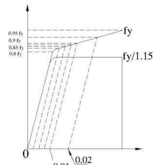
Fig 2.4 stress-strain curve for cold worked deformed bars
