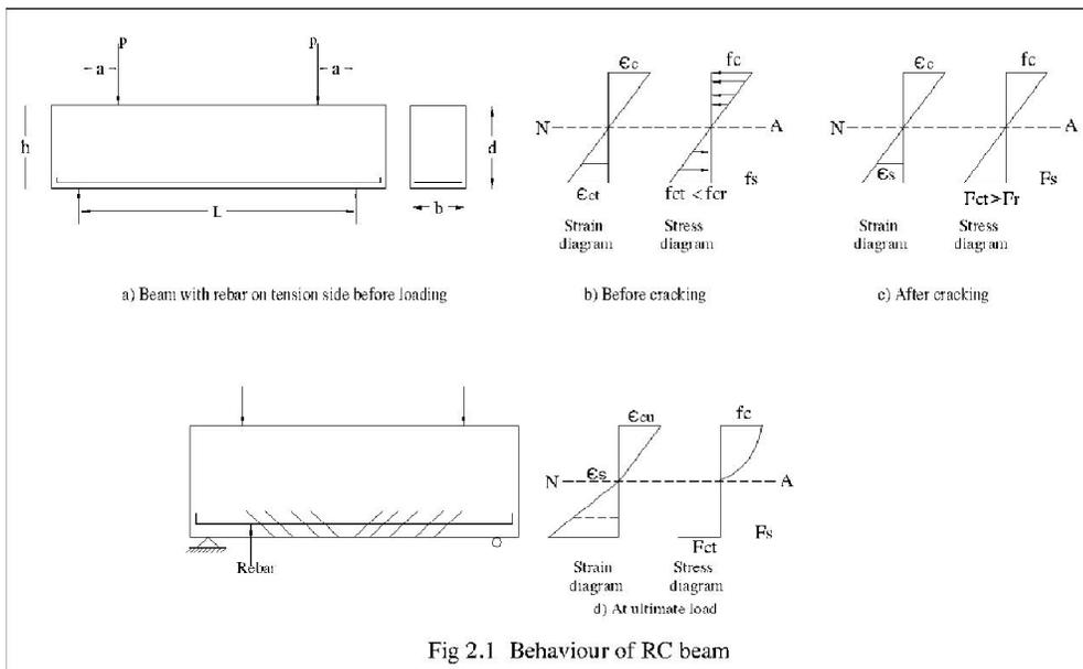
When the load is gradually increased from zero to the ultimate load value, several stages of behavior can be observed. At low loads where maximum tensile stress is less than modulus of rupture of concrete, the entire concrete is effective in resisting both compressive stress and tensile stress. At this stage, due to bonding tensile stress is also induced in steel bars.
