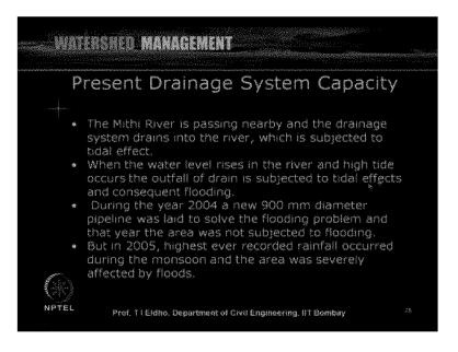
Here the two issues are there: one is the main flow taking place within the area and then also the tidal rise, what is happening within this river system. Then, that will be the back flow coming to the area. When the water level rises in the river and high tide occurs, the outfall of drain is subjected to tidal effects and consequent flooding. During the year 2004, a new 900 mm diameter pipeline was been constructed, but in 2005 as I mentioned, again there was flooding.
