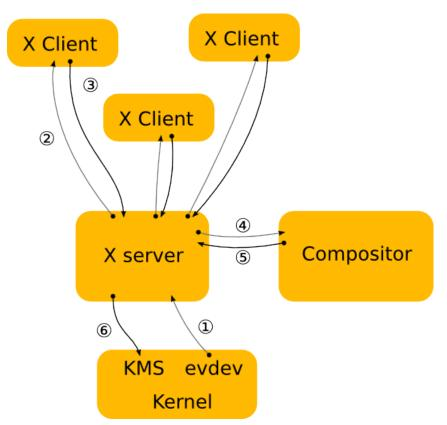
The diagram above illustrates the central role of the X server and compositor in operations, and the steps required to get contents on to the screen.
