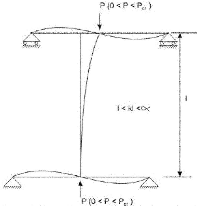
**Fig.10.27.6:** Column partially restrained at both ends
