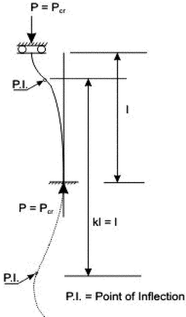
**Fig. 10.27.5:** Column rotationally fixed at both end, ( $k = 1$ )
