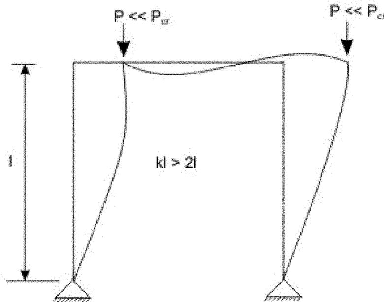
**Fig. 10.27.8: Unbraced portal frame ( $k > 2$ )**
