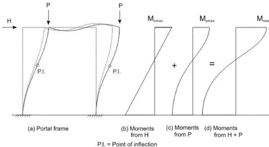
**Fig. 10.27.13:** Fixed portal frame - laterally unbraced
