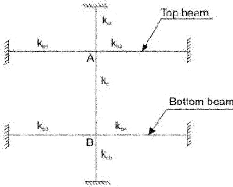
**Fig. 10.27.16:** Stiffness of columns in Wood's chart
