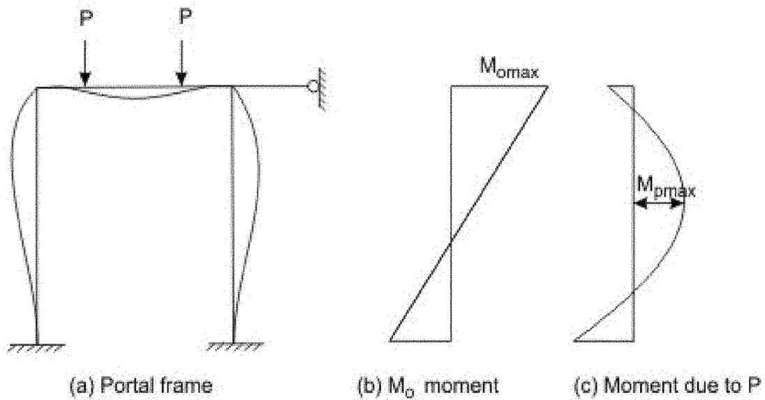
**Fig. 10.27.14: Fixed portal frame - laterally braced**
