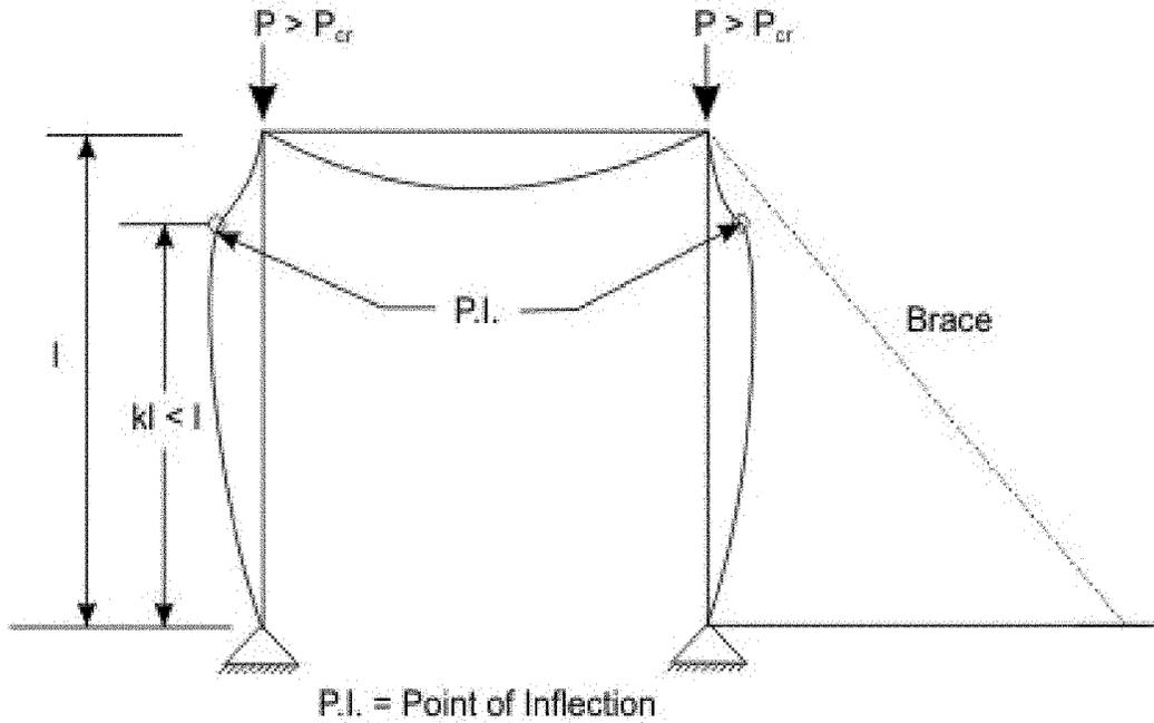
**Fig. 10.27.7: Braced portal frame ( $k < 1$ )**
