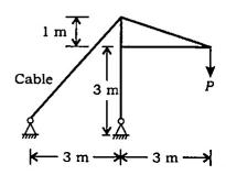
In the simple system shown in the figure, the load P is equal to 4 tonnes. What is the tension in the cable?
