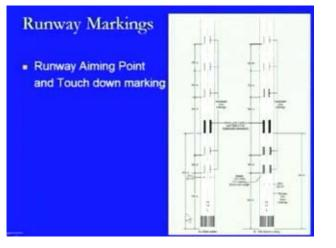
So, starting from these 4 lines which are provided to the single line, which is being located up to this particular distance, as we are providing them, that is the runway touch down zone. So, the aircraft will be coming and will be touching at this location and these strips are provided depending on the requirement; this number will be changing. There will be four four strips and then, the three three strips and so on.
