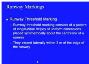
way it is provided. Generally, these are 90 centimeter wide. This is the most general width which is used for the strips.
