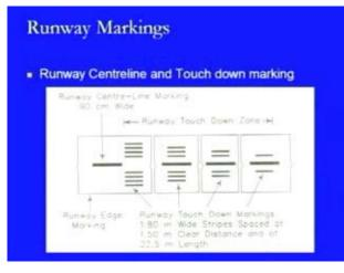
basically define the way the aircraft has to move and by what particular point afterwards only the touch down can be done. So, therefore there will be a zone in which this touch down will be made.
