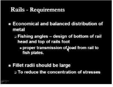
If they are not getting fitting in then there will remain some gap between the fishing plates and the web of the rail section and because of that there will not be proper transmission of load from rail to the fish plates. So the location at which the head is connected to the web or the foot is connected to the web at that point whatever curvature have been provided at that level the fishing angles have to be designed in that form so that the proper connectivity is maintained.
