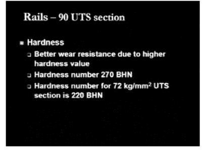
The 90 UTS rail section is having hardness number of 270 BHN; this is Brinel Hardness Number, as you must have studied in the previous years. This is the way of defining the hardness based on the indentation in the metal. So on the basis of that it is giving a value of 270 as a hardness number whereas in the case of 72 kg per mm square UTS rail section this value is 220 BHN, so it is quite higher as compared to that one.
