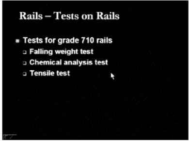
The chemical analysis test is to identify the proportion of the chemicals which have been used; the type of chemicals which have been used in the manufacturing of that rail section and the tensile test so as to identify the tensile strength of the rail section so that we can find out what are the stresses which can be taken up by that rail section. In the case of 880 rail grade there are some more test other than the falling weight test, chemical analysis test and tensile test.
