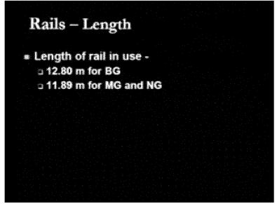
So this is length of rail sections which is used. Now this is restricted, we are not having the bigger rail section because of certain reasons. The one is that ease of manufacturing. We can easily manufacture smaller rail sections as compared to the large long rail sections
