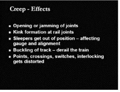
As the rail is moving it is trying to open out the joint at one end whereas it is trying to close the joint at the other end. Therefore, this is one of the effects which of the creep, that is, it will be opening the joint or it will be jamming the joint means it will just try to abort the 2 rail sections with each other and therefore the joints will not be there or there will be a problem associated with the movement of the rails with respect to the some other stresses.
