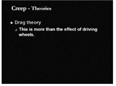
Now there are some more reasons which have been stated which cause the creep in the rail sections. The one of the reason is the starting, accelerating, slowing or stopping of the wheels.
