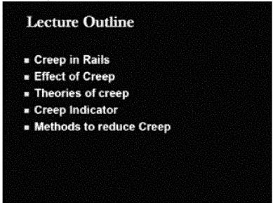
So we start with the definition of creep. The creep can be defined as the longitudinal movement of rails in a track. In the case of the rails as we seen discussed previously also they are being fastened with the sleepers using different fastenings and therefore they are assumed to be static in nature, but there are certain reasons due to which these rails start moving in certain direction and that movement in the longitudinal direction is termed as creep.
