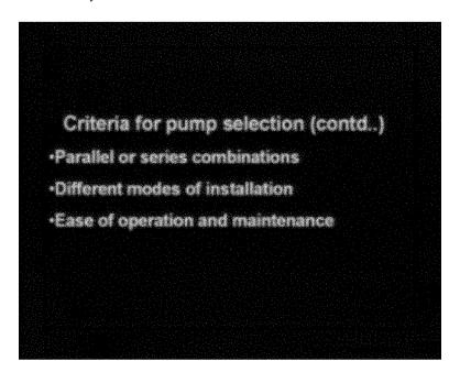
Finally we have the ease of operation and maintenance. The pumping installation should be such that we can maintain these pumping installations easily. We also have to know the kind of operation whether it is easy or difficult because many times the operators are not well qualified to be able to implement very complex operating schedule so the operation should be such that it is easy to operate the pump and it is easy to maintain and pump selection many times is based on that criteria.
