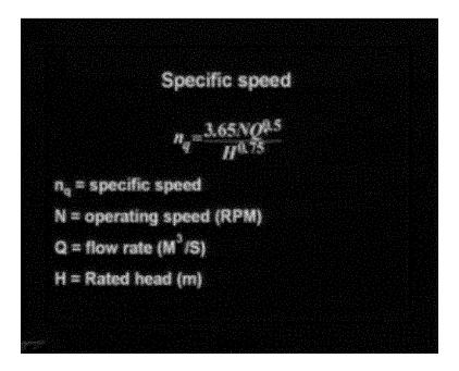
So, if you see the specific speed for the same pump given by another number you should understand that the person is using a different unit system. this is the unit system that we use for defining specific speed in our country or this is the one which is recommended by our water supply manual, our water supply and treatment manual given by the water
