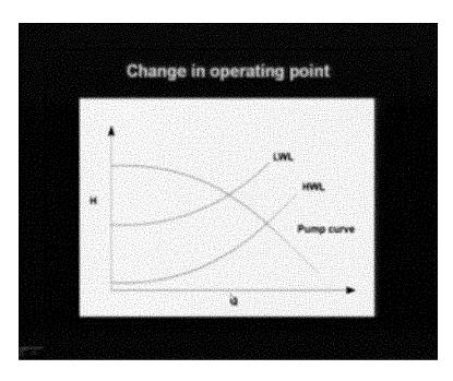
When the water level in the pump is very low then the static lift increases and when the pump is operating under such conditions you will get a low discharge to balance for the high head. Whereas when we have high water level in the sump then the static lift is reduced and to compensate for reduced total head the discharge will increase. So the pump will be operating between this operating point and this operating point during the operation corresponding to low water level and high water level.
