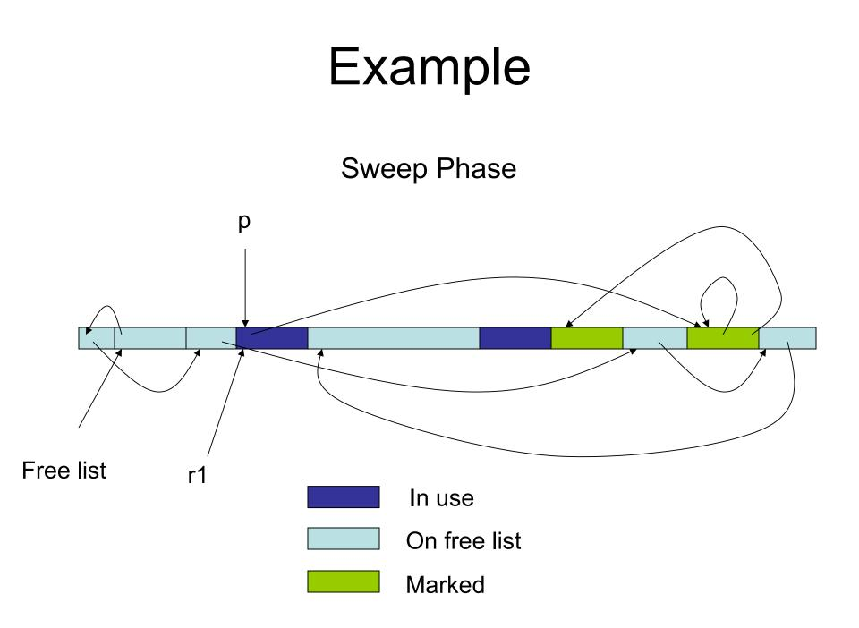
Sweep Phase: GC complete when heap boundary encountered; resume program
