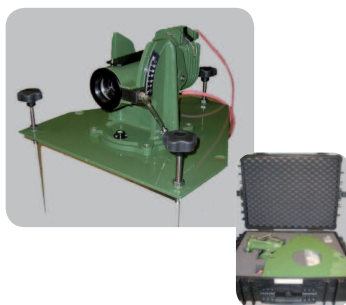
PGPI Portable glide path indicator
