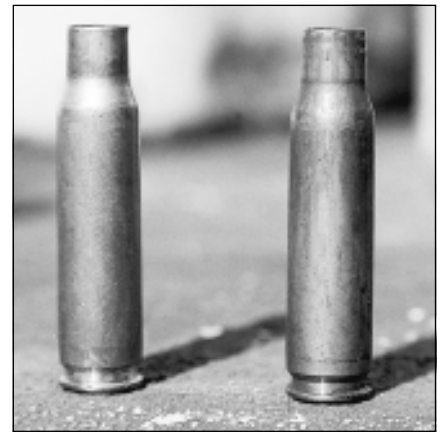
The G3 case (right) compared to a normal fired case. Note the flutes and "smoked-up" appearance.
