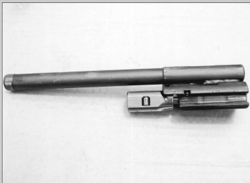
The G3 working parts. Note the roller locking lugs.
