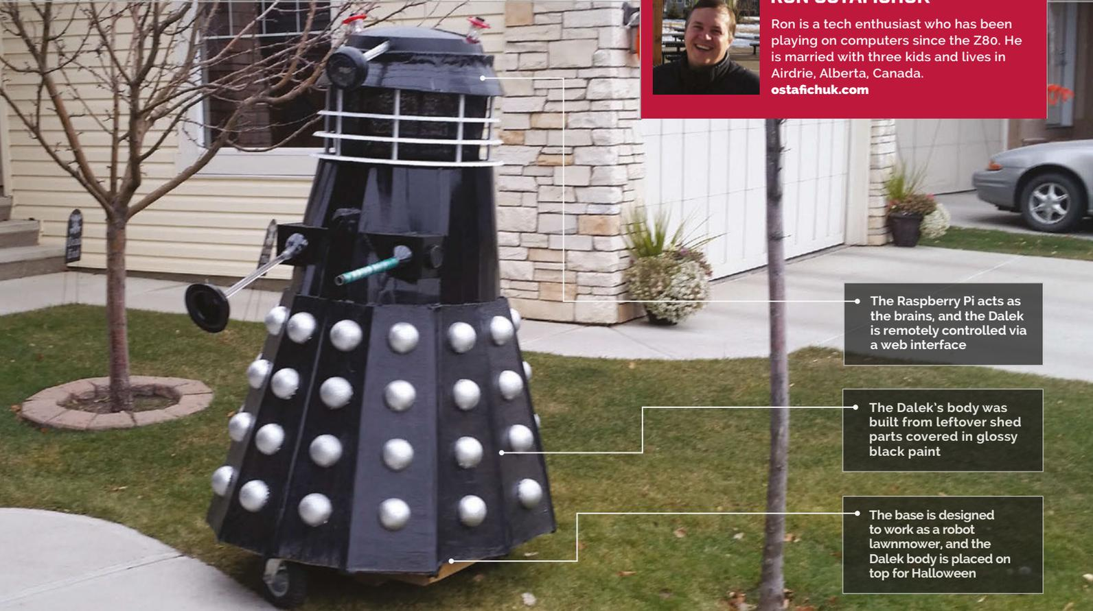
• The Raspberry Pi acts as the brains, and the Dalek is remotely controlled via a web interface
