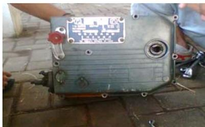
Gambar 2. Tutup *timing gear*
