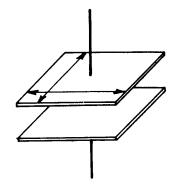
CAPACITANCE VARIES WITH THE TYPE OF INSULATING MATERIAL USED
