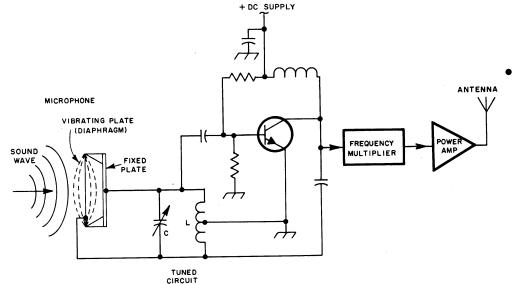
Schematic diagrams include all the individual components and how they are connected.
