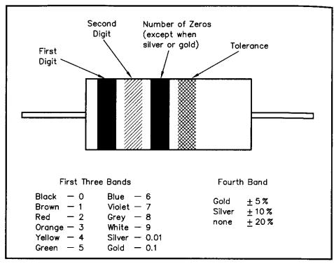
Figure 6-23 — Small resistors are labeled with a color code to show their value. For example, proceeding from left to right, a resistor with color bands of yellow/violet/ brown/gold is a 470- $\Omega$  resistor with a 5% tolerance.
