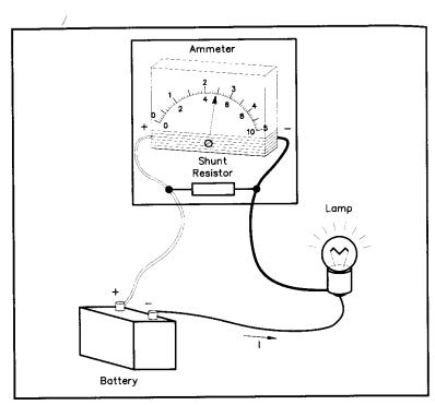
Figure 4-13—To measure current you must break the current at some point and connect the meter in series at the break. A shunt resistor expands the scale of the meter to measure higher currents than it could normally handle.
