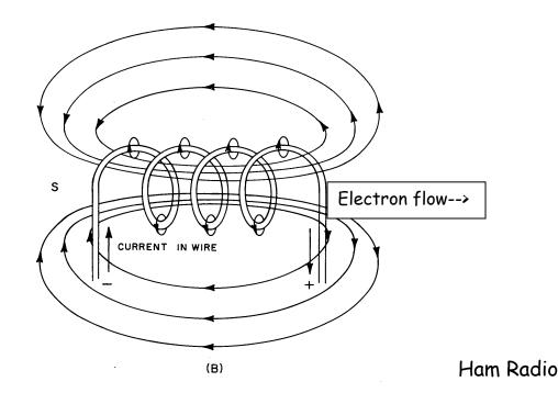
Note: current flows from + to -, but is carried by electrons which flow from - to +
