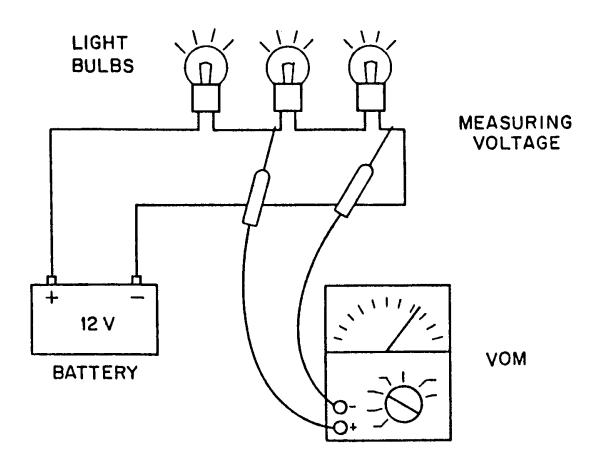
Voltmeter measures across the circuit (in parallel to the voltage to be measured)
