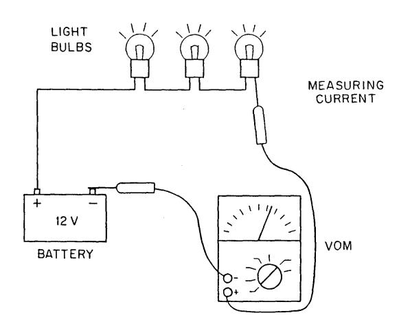
Ammeter must be part of the circuit to measure the current
