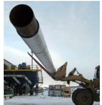
Pre-Insulated Pipe: Pyrogel enables pre-insulation and subsequent transport of pipe.
