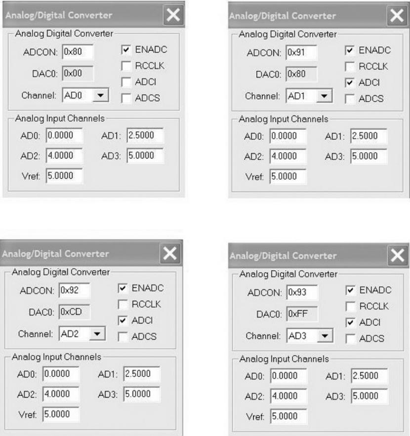
**Figure 5.11** Analog/digital converter window showing values for channels AD0, AD1, AD2 and AD3
