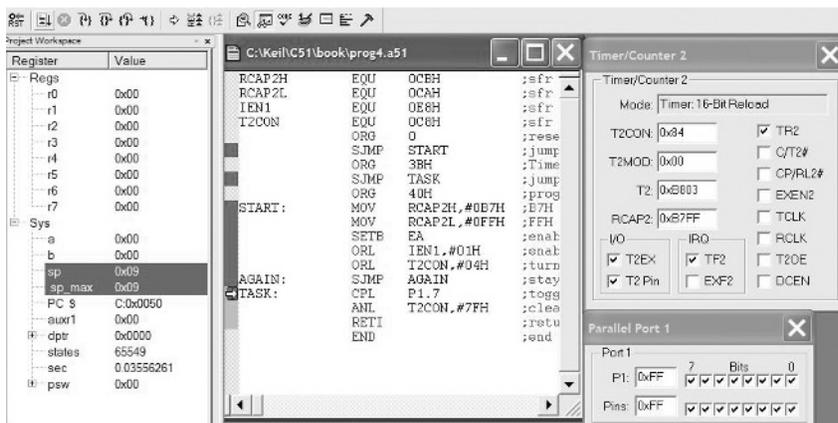
**Figure 4.12** Simulation display with breakpoint used to determine timing
