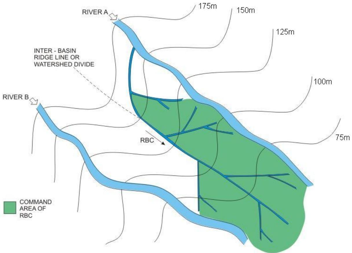
FIGURE 5 : Command area for a typical canal system
