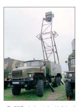
The ELINT system's control post is designed to define planar coordinates and motion parameters of radio emitting sources based on data provided by the three stations, as well as to couple with the superior control centre.
