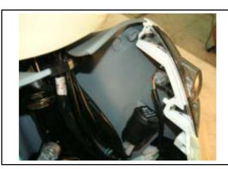
Turn left and pull out the bulb seat.
