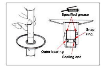
Install a new inner bearing.
