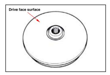
Install movable drive face assembly onto crankshaft.
