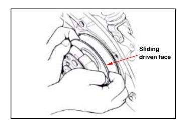
Install the clutch set with drive belt onto the drive shaft.
