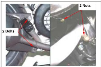
Remove the air cleaner connection bolts (2 bolts).
