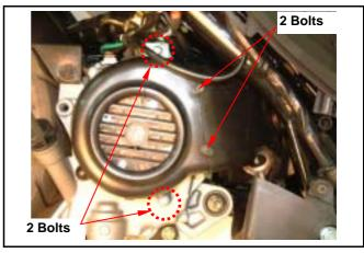
Remove the cooling fan (4 bolts).
