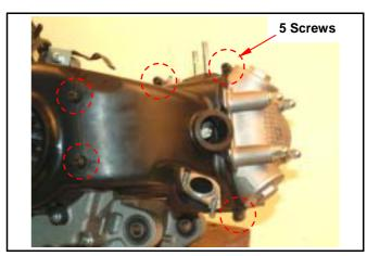
Install the engine onto the frame. (Refer to chapter 5)
