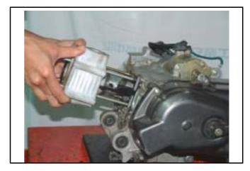
Install the cam chain plate, the cylinder gasket and lock pins.
