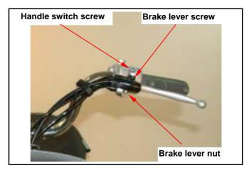
Remove left handle screw and cable clamp. Remove the left handle switch.
