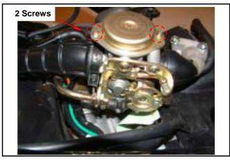
Remove compress spring and vacuum piston.
