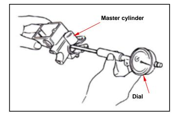
Measure the outer diameter of the piston. Replace the piston if its measured value exceeds allowable limit.
