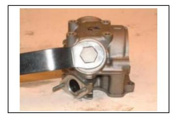
Remove the camshaft stopper of the rocker arm shaft (1 bolt).
