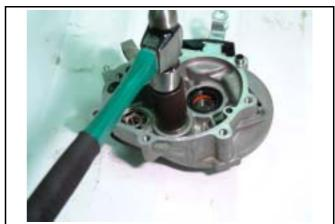
Press out the drive shaft from the gear box cover. Remove oil seal from the gear box cover. Remove the drive shaft bearing from the gear box cover with the inner type bearing puller.
