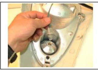
Front Turn Winker Light Bulb Replacement Remove the front cover. (3 screws)
