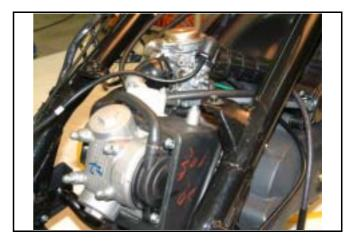
Remove the exhaust muffler (2 Bolts, 2 Nuts).
