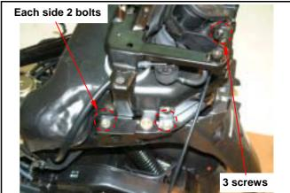
Turn fuel unit setting plate to the left, and then remove fuel unit.
