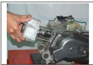
Remove cylinder gasket and lock pins.
