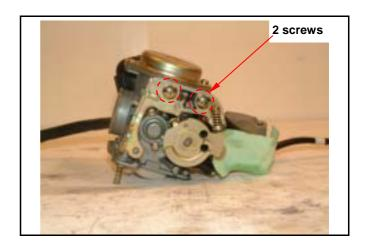
Remove the screws (screw x 2) of the air cut-off valve and its cover.
