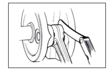
Measure the radical clearance of the big end at the vertical directions.
