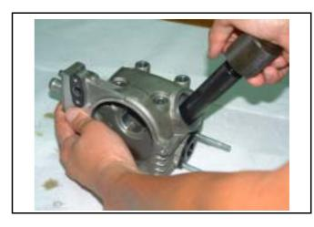
Tap valve stem with a plastic hammer to make valve retainer and valve stem sealing properly.
