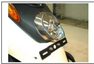
Push and turn left the bulb, and then remove the bulb.
