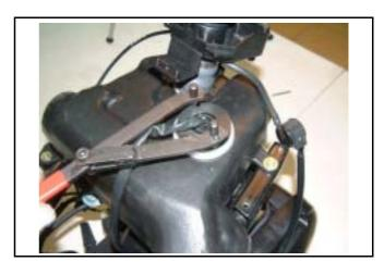
Check if the float and washer is damaged. Replace it with new ones if damaged.
