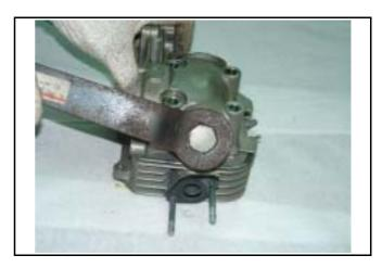
Remove the camshaft stopper of the rocker arm shaft (1 bolt).
