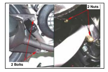
Remove the fan shroud (2 screws, 2 bolts).
