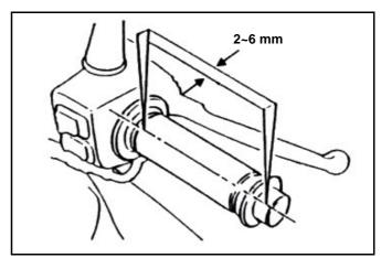
Adjustment can be done in either ends. Secondary adjustment is conducted from top side. Remove rubber boot, loosen fixing nut, and then adjust it by turning the adjustment nut.
