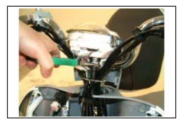
Disconnect the instrument panel and switch wiring couplers.
