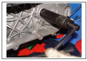
Install new oil seal with the special service tool.
