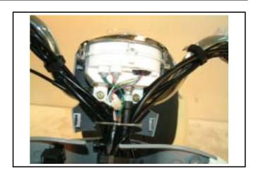
Remove meter mounting screws (3 screws), and then remove meter.
