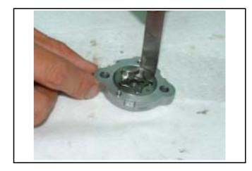
Check clearance between inner and outer rotors.
