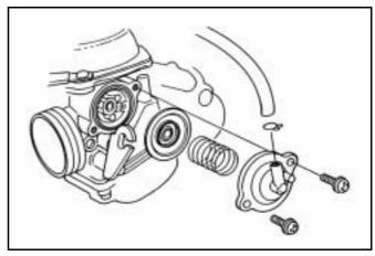
Remove the spring and vacuum diaphragm. Check if the diaphragm for deterioration or crack.
