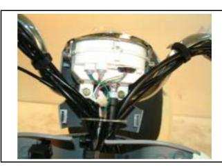
Pull out the bulb and replace it with new one.
