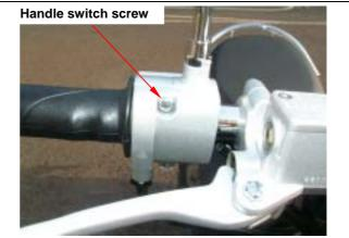
With a wrench to hold the handles bolt and then remove the nut.
