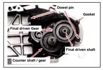
Install the dowel pins (2 pins) and new gasket. Install the gear box cover and 7 bolts (tighten the bolts).
