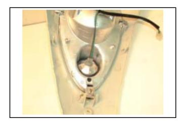
Pull out the bulb and replace it with new one. (12V/10W)
