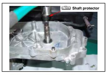
If the driving shaft is pulled out with its bearing, then remove the bearing with bearing puller and bearing protector.
