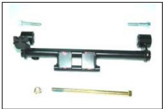
Check if the engine hanger bush and cushion rubber for damage. If so, replace with new ones.
