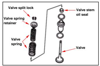
Install the valves with the valve remover/installer. **Special Service Tool:**
