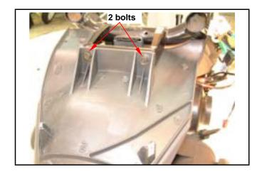
Remove the 2 bolts on the two sides. (1 bolts on each side).
