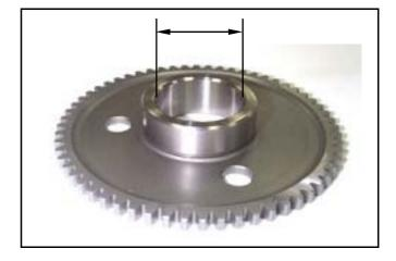
Check the starting idle gear and shaft for wear or damage.
