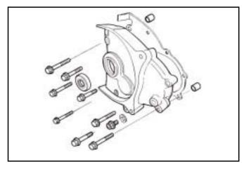
Remove counter shaft and gear. Remove final driven gear and shaft. Remove gasket and dowel pins.
