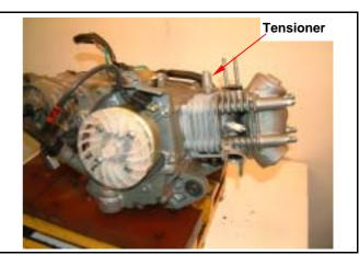
Remove the cylinder head side cover. (2 bolts)
