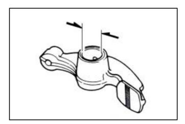
Measure the active O.D. of the cam rocker arm shaft and cam rocker arm.
