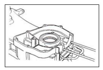
Install crankshaft into the left crankcase and then install two and new crankcase gasket.
