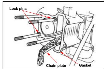
Tighten the cylinder head nuts (4 nuts)
