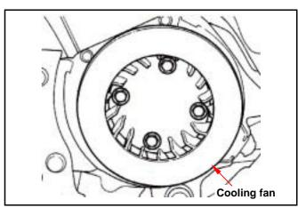
Hold the flywheel with the universal fixture. Remove the 10mm nut on the flywheel. Special Service Tools:
