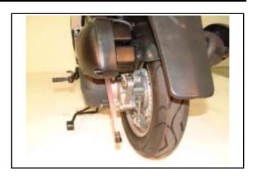
Remove gear oil filling hole bolt and place a measurement cup under the draining plug. Remove the oil draining plug and the pour gear oil into the measurement cup. Measure the gear oil quantity if within standard value. Add specified gear oil if the oil level too low.
