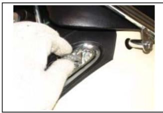
**Bulbs Replacement of Speedometer** Remove the handle front cover. (3 screws)
