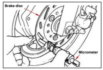
Remove the brake disc from wheel. Check the disc for deformation and bend.
