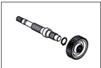
Check bearings on gear box and cover. Rotate each bearing's inner ring with fingers. Check if bearings can be turned in smooth and silent, and also check if bearing outer ring is mounted on gear box & cover tightly. If bearing rotation is uneven, noising, or loose bearing mounted, then replace it. Check oil seal for wear or damage, and replace it if necessary.
