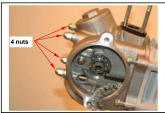
Remove the cylinder head. Clean up residues from the matching surfaces of cylinder and cylinder head.
