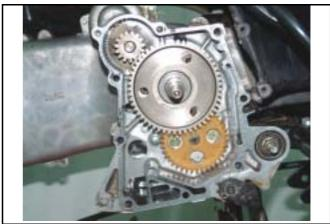
Hold the starting driven gear with the universal fixture.
