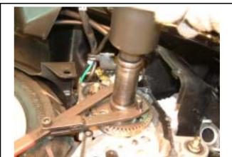
Remove starting clutch, starting idle-gear, and shaft.
