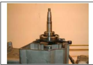
Slightly shake the crankshaft and then remove it and the chain.
