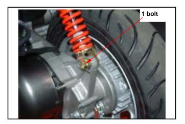
Remove the engine hanger nuts and bolts (engine side), and then remove the engine.
