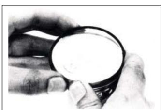
Install the piston rings and then measure clearance between piston ring and its grooves. Service Limit: Top ring: replace if over 0.09mm 2<sup>nd</sup> ring: replace if over 0.09mm
