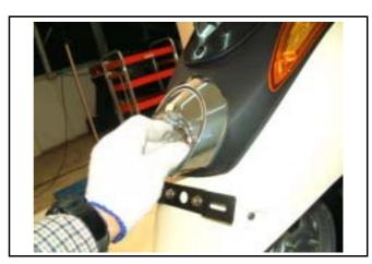
Replace the bulbs of the tail light, brake light (12V 5W/18W).
