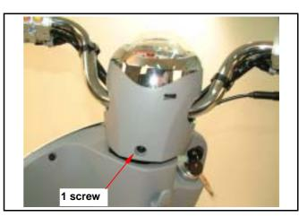
Remove meter mounting bolts (2 bolts). Remove handle rear cover and meter.
