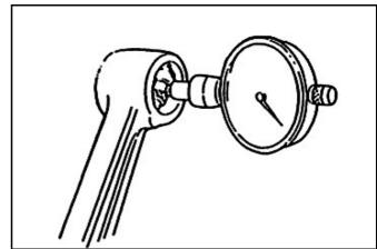
Measure the inner diameter of piston pin hole. Service Limit: (Refer to page 2)
