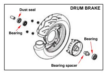
Remove the bearing with the inner type bearing remover.
