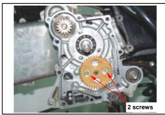
Install oil pump drive gear.
