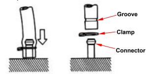
Rubber and plastic boots should be properly reinstalled to the original correct positions as designed.
