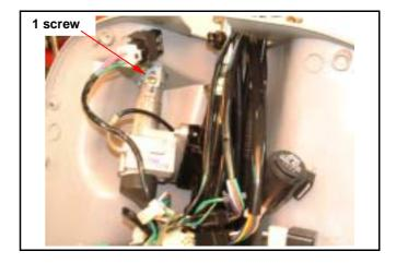
Remove the rear mounting screw (1 screw) of the inner cover.
