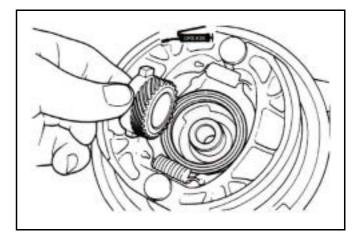
Align the flange part on the speedometer gear with the slot of wheel hub, and then install the brake disc (drum brake) or speedometer gear box.
