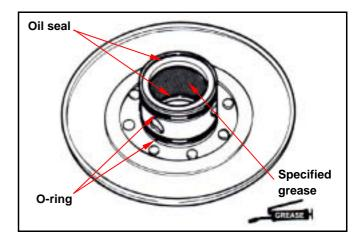
Install sliding driven face onto driven face. Install guide pin and guide pin roller.
