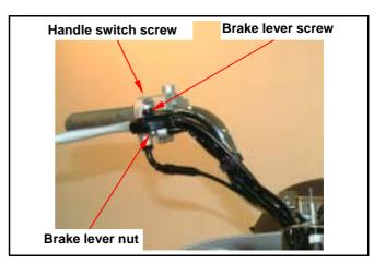
Remove right handle screw and cable clamp. Remove the right handle switch, throttle cable.
