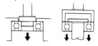
Both of these examples can result in bearing damage.
