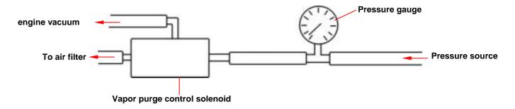
2) Apply 100mmAq into pressure source inlet as engine stopped then plug it. The pressure at the gauge should not drop to below 10mmAg within 10 seconds.
