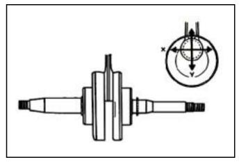
Place the crankshaft onto a V-block and measure run-out of the crankshaft with dial gauge. Service limit: Replace when it is more than 0.10 mm.
