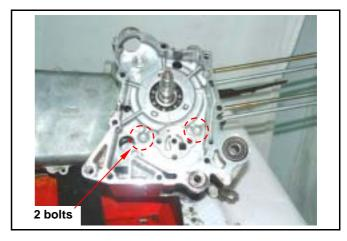
Install the cam chain tensioner.
