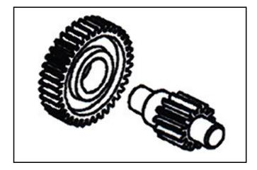
Check if the final driven shaft and gear are wear out or damage.
