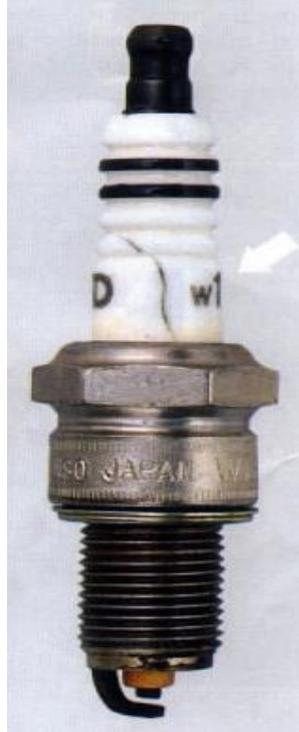
**Gambar 2.45: isolator busi pecah (tanda panah)**
