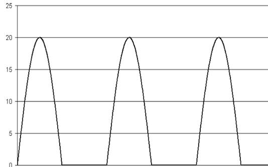
This isn't DC... but the diode has removed all of the negative-going parts of the waveform.
