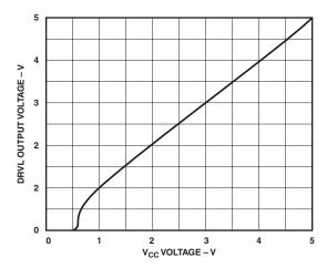
TPC 9. DRVL Output Voltage vs. Supply Voltage
