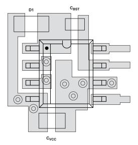
*Figure 5. External Component Placement Example for the ADP3418 Driver*
