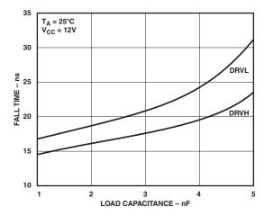
TPC 6. DRVH and DRVL Fall Times vs. Load Capacitance
