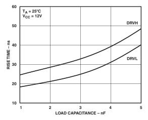
TPC 5. DRVH and DRVL Rise Times vs. Load Capacitance
