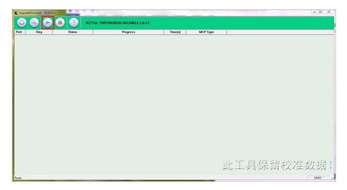
5. Remove the battery from device. **HOLD the VOLUME minus button**, **connect cable from the computer**, **plug in battery**. The device is loaded automatically
