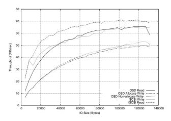
Figure 7. Raw performance comparison of OSD and iSCSI
